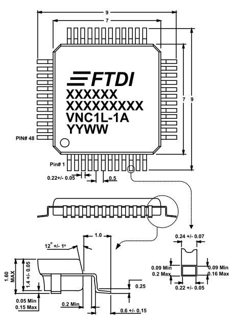
Figure 9 - LQFP-48 Package Dimensions
