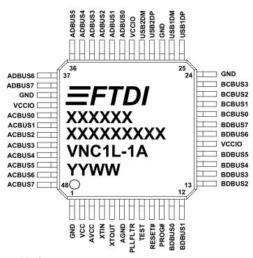
Figure 2 - 48 pin LQFP Package Pin Out
