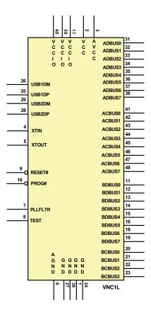
Figure 3 - VNC1L Pin Out - Schematic
