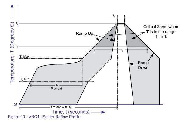
The VNC1L is supplied in Pb free 48 LD LQFP package. The recommended solder reflow profile is shown in below.
