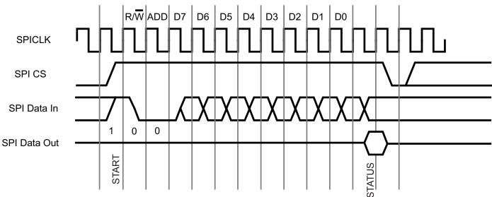
From Start - SPI CS must be held high for the entire write cycle, and must be taken low for at least one clock period after the write is completed. The first bit on SPI Data In is the R/W bit - inputting a '0' here allows data to be written to the chip. The next bit is the address bit, ADD, which is used to indicate whether the data register ('0') or the status
